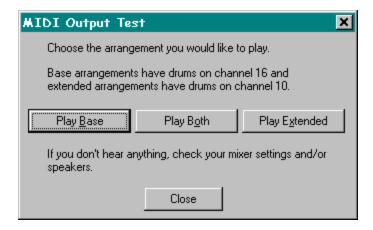
Note that the SoundCheck diagnostic program bypasses the MIDI Mapper (unless the MIDI Mapper itself is being tested) and plays the file according to the parameters set by the device. This allows you to differentiate between incorrect MIDI Mapper settings and device driver problems.
