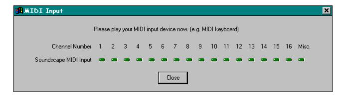
As you play the sequencer or any other MIDI device connected to your system, one or more of the LED's will light to indicate which MIDI channel is in use.
